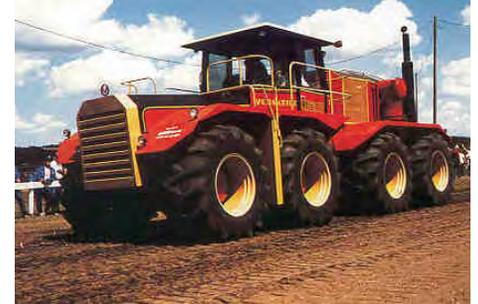
Big Roy was built by Versatile in 1977 at its plant in Winnipeg. The largest tractor ever built the Versatile 1080 (Big Roy) was actually too heavy to use as its tires compacted the soil too much. They tried to alleviate this by tripling the number of wheels. The result was a tractor with 24 wheels that was nearly impossible to turn.
